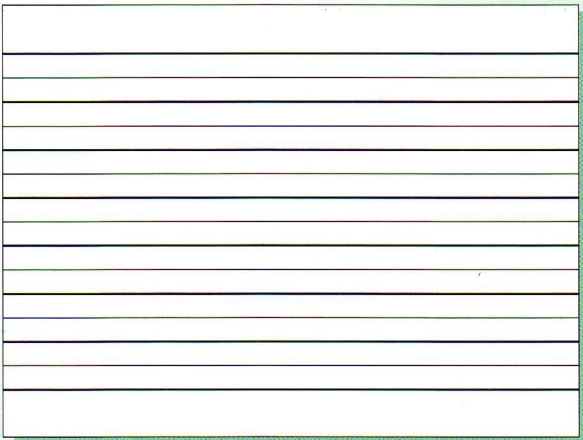
Alternating 1/16" (1.58 mm) and 1/32" (.79 mm) lines. 2" (50.8 mm) line spacing, 4" (101.6 mm) border, top and bottom.
