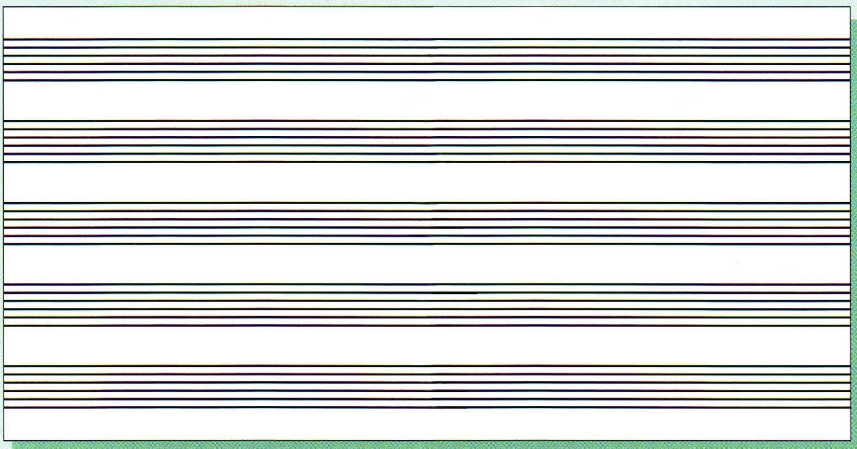
Five 1/16" (1.58 mm) lines per section. 1" (25.4 mm) line spacing, 5" (127 mm) between sections. 4" (101.6 mm) border, top and bottom.
